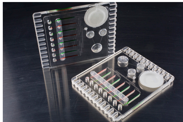
Above: Plastic (PMMA) analysis chip with dried reagents for up to six virus-specific RT-LAMP assays, plus controls.
