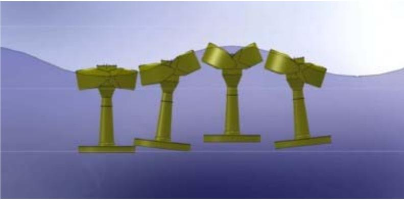
Figure 5: Representation of a prior generation of the Columbia Power Technologies Manta device. [<http://www.columbiapwr.com/rayseries.asp>]
