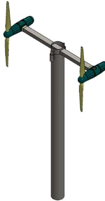
Figure A-1. Dual-rotor axial-flow tidal turbine
