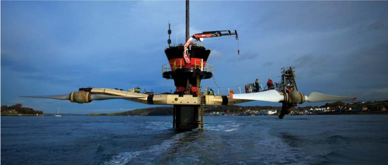
Figure 6: The SeaGen axial flow tidal turbine above water, ready for onsite maintenance
