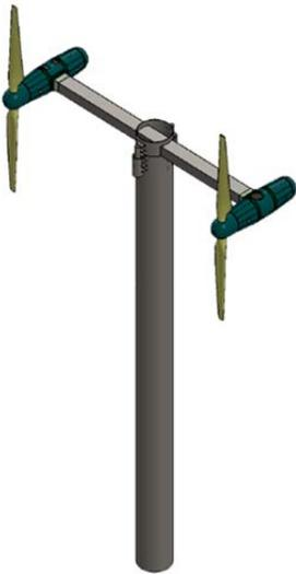
Figure 2: An illustration of the dual rotor axial flow turbine assessed in RM1.
