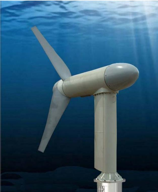
Figure 5: An Illustration of Verdant Power's axial flow tidal turbine.
