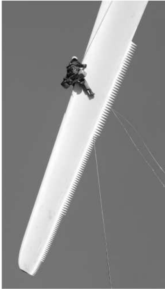
Figure 2. Trailing edge serrations on the blade of a GE 2.3 MW prototype turbine. From [1]. Reprinted with the author's permission.
