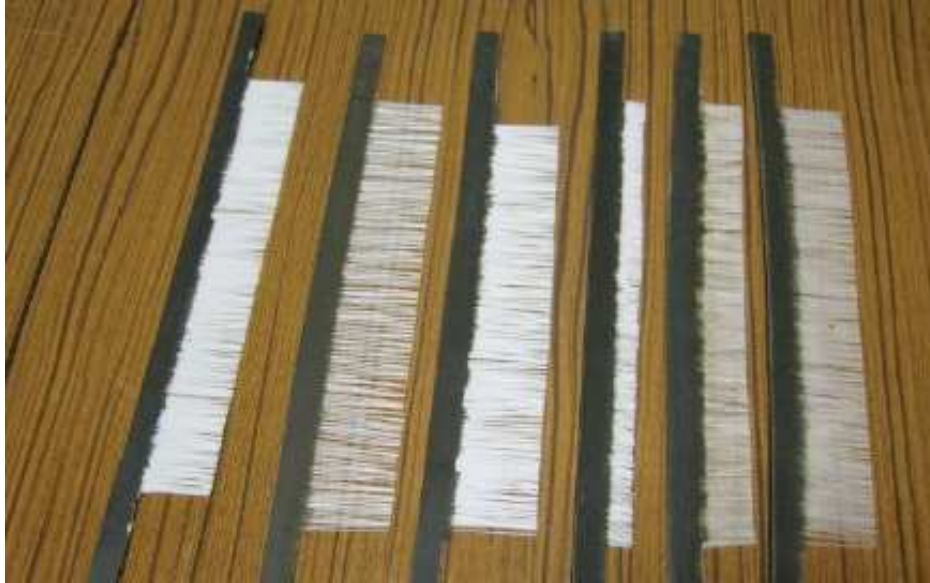
Figure 3. Trailing edge brush attachments. In this photograph, each brush consists of a single row of polypropylene fibers. From [2]. Reprinted with permission of the American Institute of Aeronautics and Astronautics.
