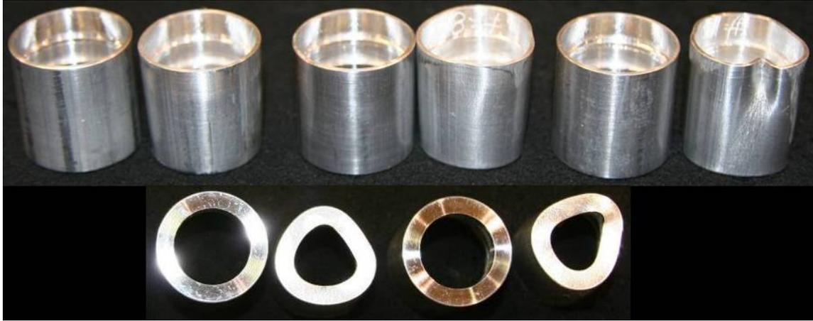
**Figure 5: Side (top) and breech (bottom) views of unfired (left) and fired (right) projectiles**
