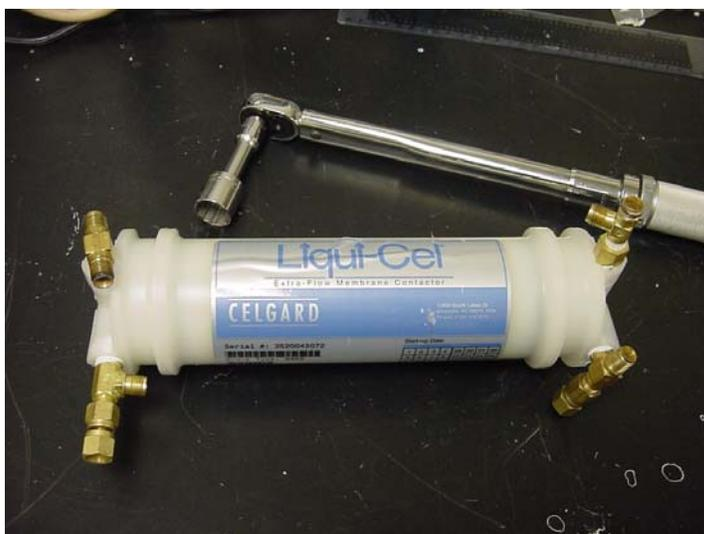
**Figure 8.** Celgard X-50 membrane contactor.
