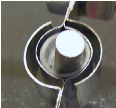
■ Figure 7. Steel rod in small Ta heater before heating
