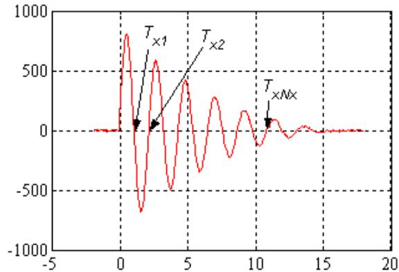
Figure 15. Measured current zero crossings.
