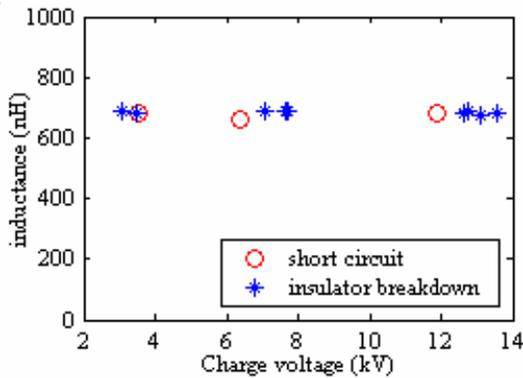
Figure 19. Estimated inductance versus capacitor charge voltage.
