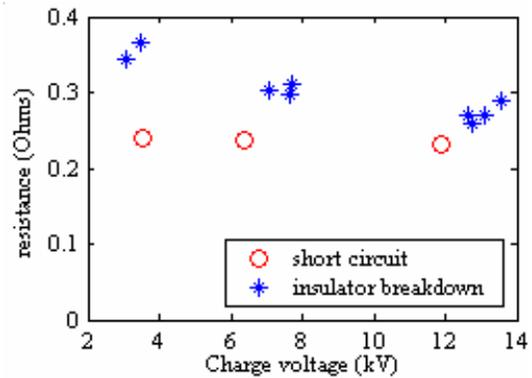
Figure 20. Estimated resistance versus capacitor charge voltage.
