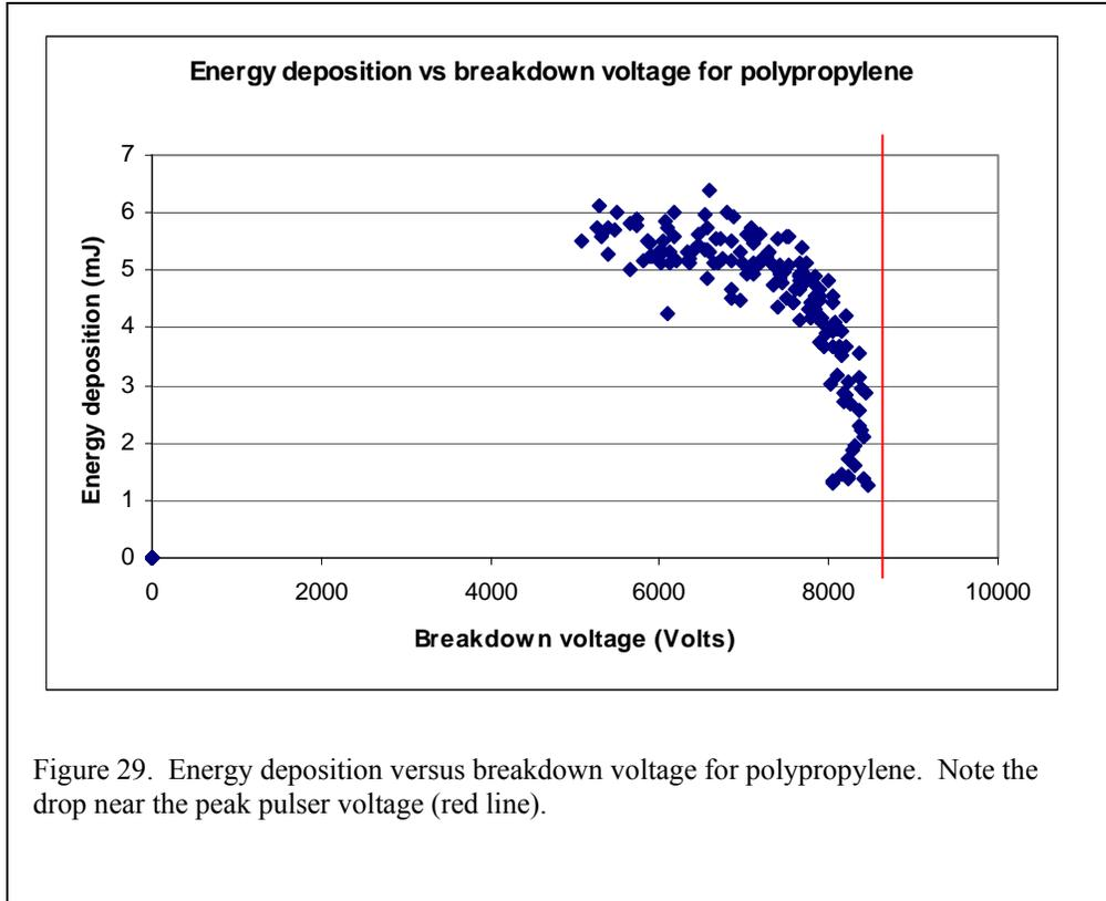
Figure 29. Energy deposition versus breakdown voltage for polypropylene. Note the drop near the peak pulser voltage (red line).
