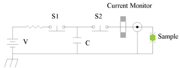
Figure 11. Schematic of high energy discharge experiment.
