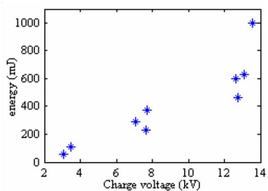
Figure 22. Estimated energy deposition versus capacitor charge voltage.
