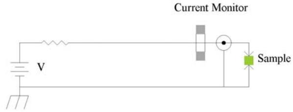
Figure 23. Schematic of low energy discharge experiment.
