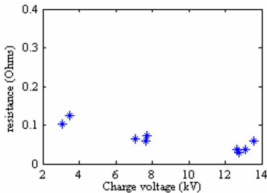
Figure 21. Estimated arc resistance versus capacitor charge voltage.
